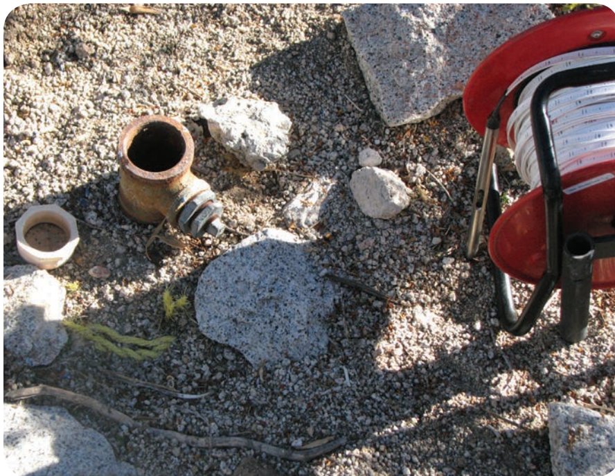
Groundwater levels are one of the most important types of data to collect. Equipment shown is a Solinst water level indicator.
